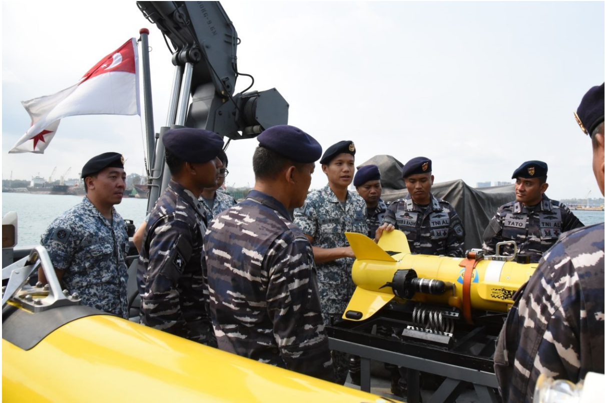
RSN personnel giving a brief on the K-STER C Expendable Mine Disposal System to TNI AL personnel on RSS Bedok.
