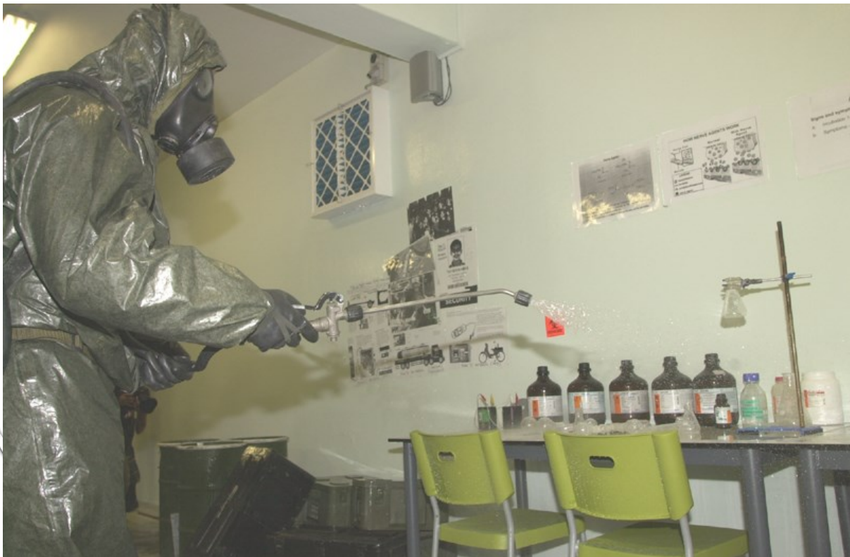
CBRE personnel using a Decon Sprayer (DS 10) to neutralize a chemical spill.
