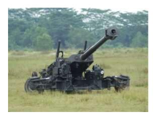
The Singapore Light Weight Howitzer Pegasus is the world's first heli-portable 155mm howitzer with a self-propelled capability.
