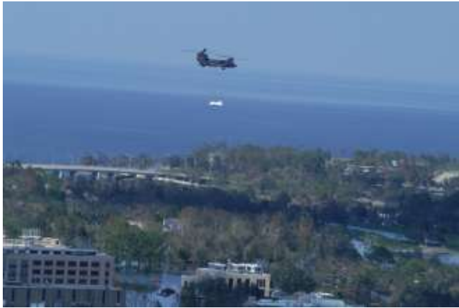
An RSAF Chinook carrying sandbags to patch a broken section of the levee separating Lake Pontchartrain from the flooded area in downtown New Orleans.
