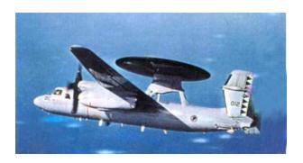
The Republic of Singapore Air Force (RSAF) E-2C Hawkeye is a sophisticated Airborne Early Warning and Control (AEW&C) platform employed to enhance air defence. It is capable of providing air and surface surveillance, as well as tactical control of air assets.
